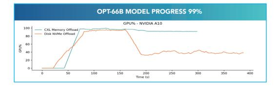
Performance of the CXL Memory Offload remained constant while Disk / NVMe deteriorated.
